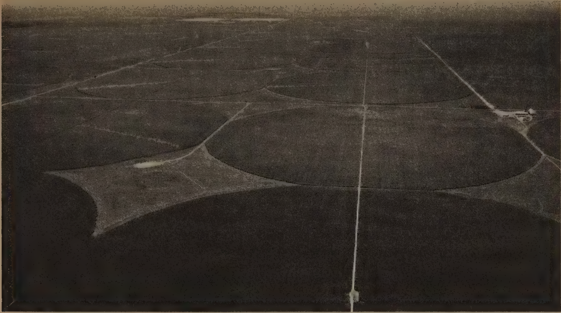
Center-pivot irrigation systems water a quarter section at a time, producing circular growing areas each a half mile in diameter.
